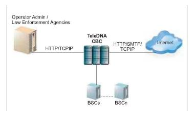
The CBC interacts with CBE (Cell Broadcasting Entity), BSCs (Base Station Controllers) of the PLMN. CBC architecture provides the fliexibility for the CBEs to connect to CBC using the GSM standarda interface.
